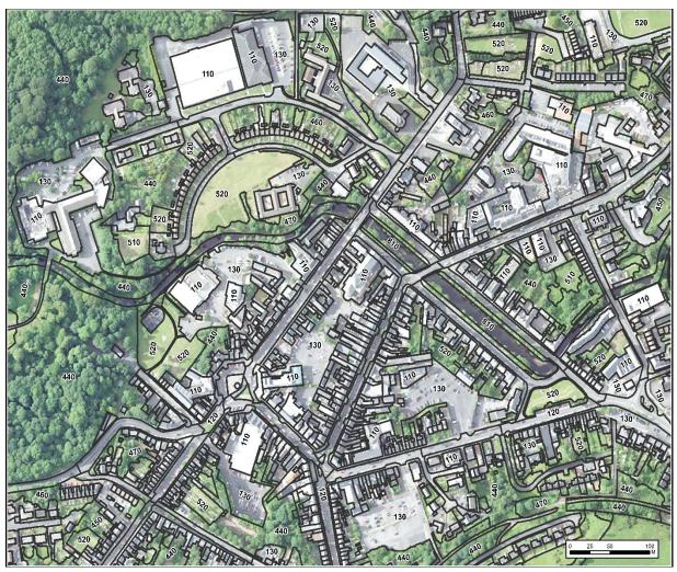
Figure 5.2: An example of the NLC 2018 map in Westport, Co. Mayo showing examples of all three Artificial Surfaces classes: Buildings (110), Ways (120) and Other Artificial Surfaces (130). Amenity Grassland (520) example can also be seen.
