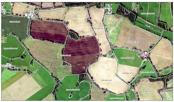
Figure 5.7: Examples of field parcels classified under the Cultivated Land Level 2 class.
