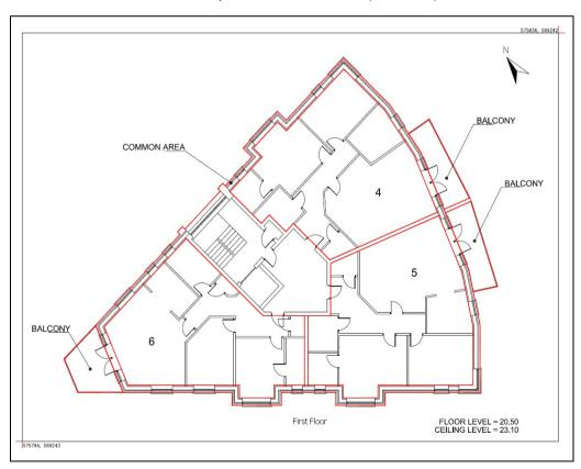
Figure 13 - Example of First Floor Plan (Block 1-11)
